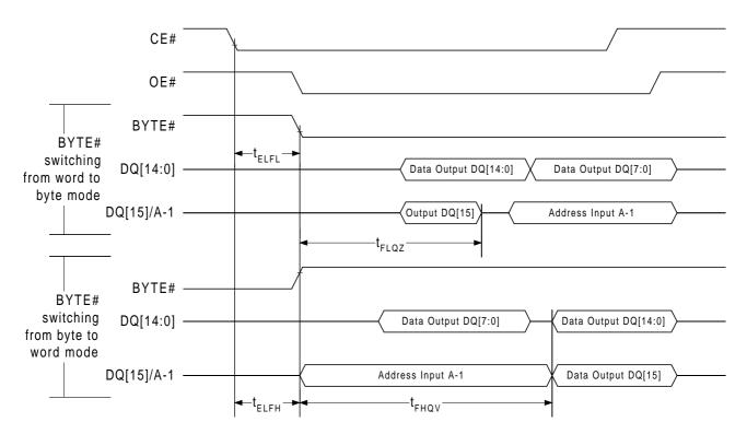
Figure 17. BYTE# Timings for Read Operations
