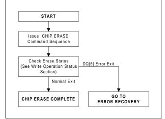
Figure 5. Chip Erase Procedure
