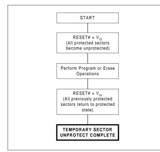
Figure 3. Temporary Sector Unprotect Algorithm
